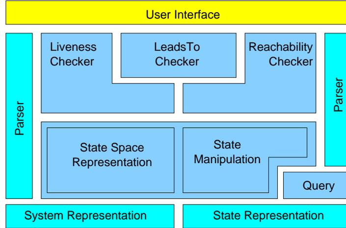
**Fig. 2.** UPPAAL uses a layered architecture. Components for representing the input model and a symbolic state are placed at the bottom. The state space representations are a set of symbolic states and together with the state operations they form the next layer. The various checkers combine these operations to provide the complex functionality needed. This functionality is made available via either a command line interface or a graphical user interface.
