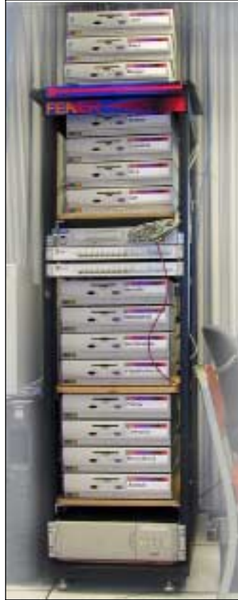
Fig. 8 — TrailBlazer Compute-Servers Fifteen standard PCs, running the Plan9 operating system as compute servers, give the TrailBlazer system a performance boost.
